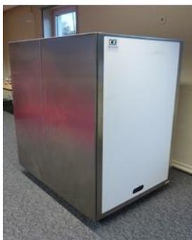
A passive stand-off mm-wave full-body scanner has been developed by **Alfa Imaging**. This deliverable presents the progress of the development work, the achieved results and the outlook for this task. Alfa Imaging had an existing passive mm-wave imager (ALFA2) that has been redesigned for XP-DITE use, increasing the aperture and improving the Automatic Threat Detection (ATD) software.
